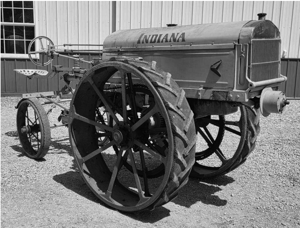
Above: This circa-1920 Indiana Tractor, built in Anderson Indiana, equipped a LeRoi 2C four-cylinder engine and chain drive, brought $21,000.
