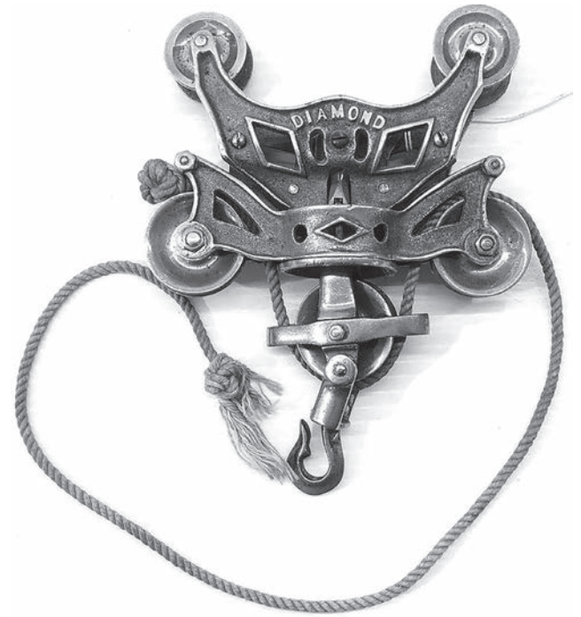
Above: A Syracuse, N.Y., Whitman & Barnes Co. overhead track hay car helped move hay from a barn floor into a top mow or loft. The pull of a rope replaced a block-and-tackle system that required several men. This sample sold for $30,000.
