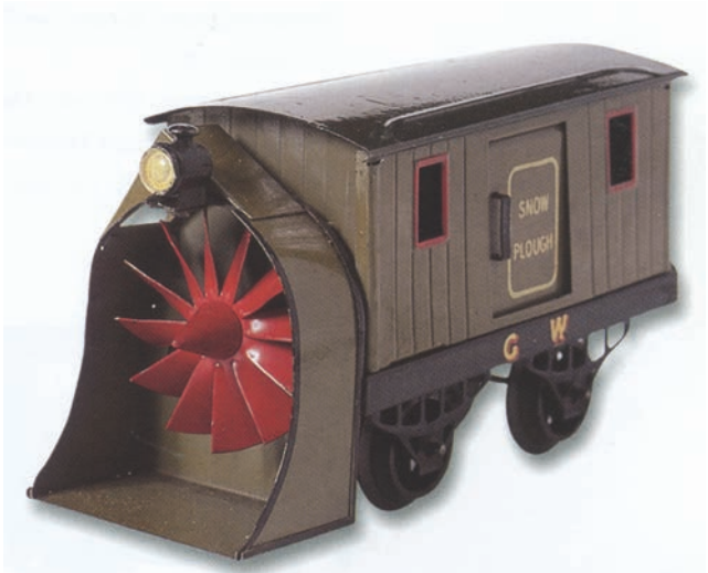
Above: The popular “Snowplough” illustrates the diversity of Hornby accessories. The Snowplough, molded after one used by Great Western Railway, was first manufactured in 1924. The fan operated by a drive belt connected to the front axle. The fan would literally “blow” snow off the tracks, keeping the tracks clean.
