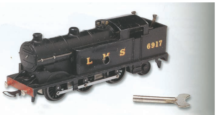
Above: Hornby "clockwork" Class 69 locomotive No. 6917 with key. Clockwork trains utilized an internal, wind-up spring and complex series of gears for propulsion. These model trains are highly collectible.
