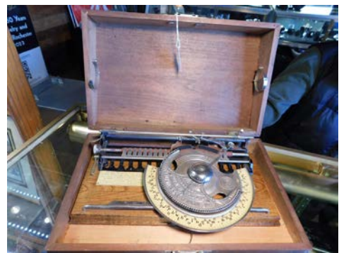
Above: Still sitting in the original carrying case, this typewriter from 1892 was meant to be used with the "hunt and peck" method.
