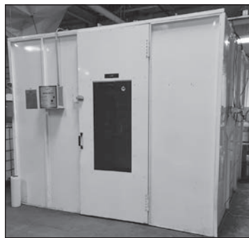
Paint Mixing Booth
