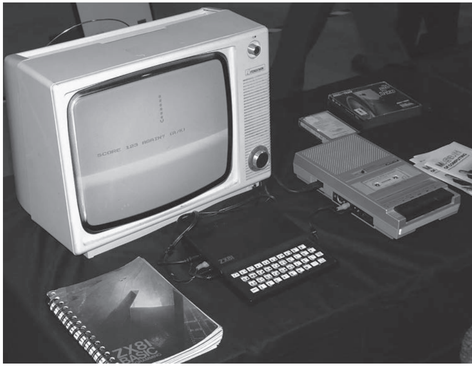
Above: This Timex/Sinclair computer is shown with an external cassette recorder/player for running programs and capturing data. They are rare, often priced around $100.
