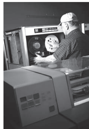
Above: Even huge mainframe computers needed a form of permanent storage. One of the first was reel-to-reel magnetic tape.
