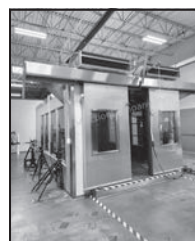
Climatic Chamber with HVAC System
