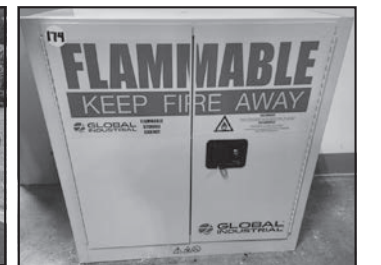
Flammable Metal Storage Cabinet
